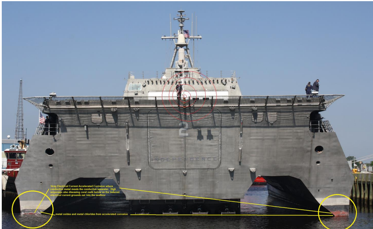
Figure 4: Accelerated stray electrical current corrosion attacked this vessel in a short period of time due to high power, high gain radars and antennas
